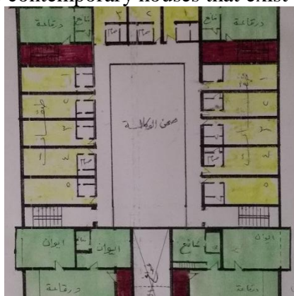
(fig. 2) the upper floor consists of: Single rooms for single trader's accommodation, the inner courtyard, hotel suites are composed of several rooms, a lounge, utilities and services.
