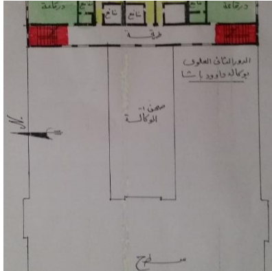
(fig. 3) the second floor consists of 3 Single rooms for single trader's accommodation, the inner courtyard, hotel suites are composed of several rooms, a lounge, utilities and services
